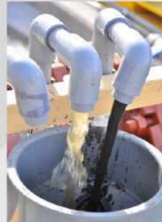
Feed Sludge and Filtrate
