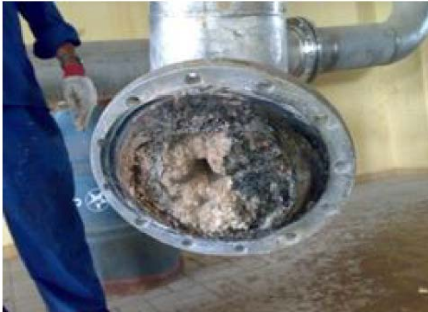
Fig. 1. Clogging of a post digestion pipe by struvite at a treatment plant (location confidential)
