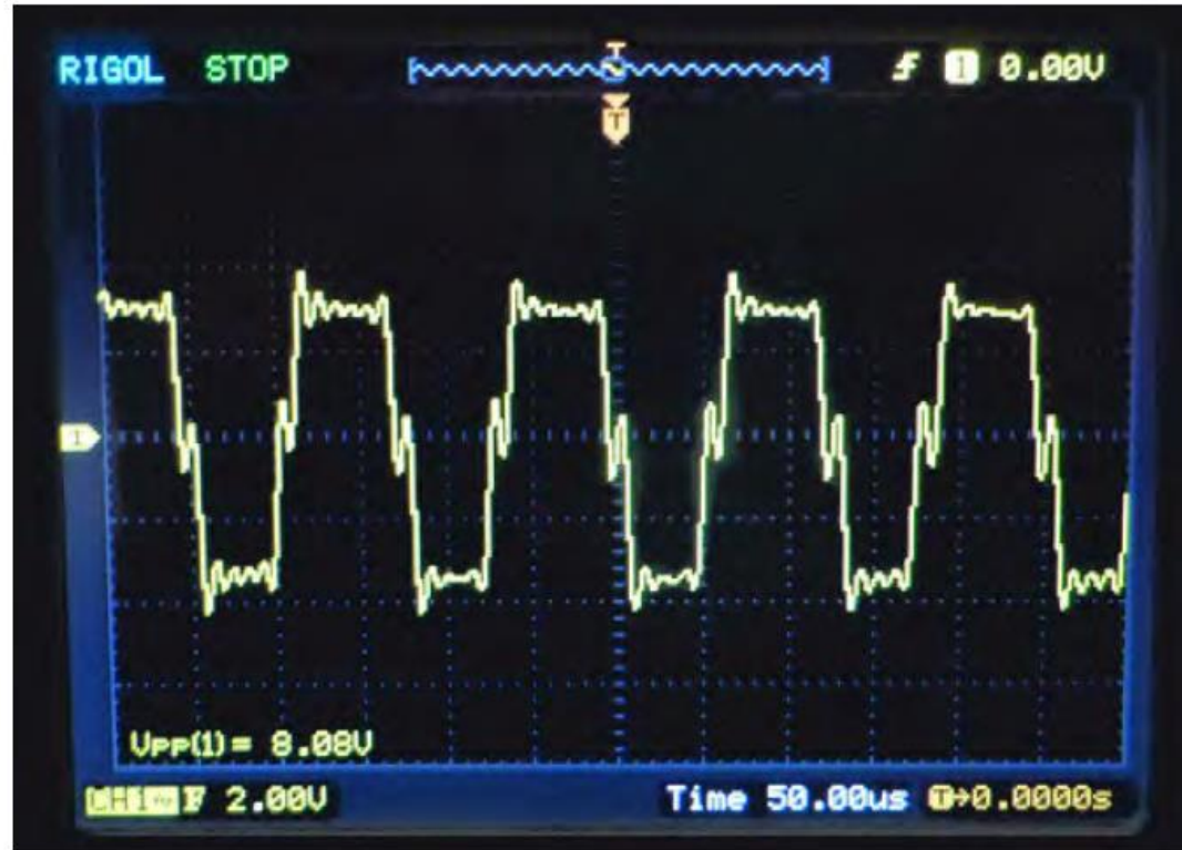
Shaft Voltage Unprotected
