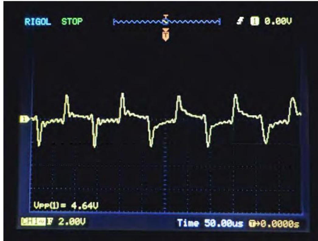
Shaft Voltage with Fiber Ring
