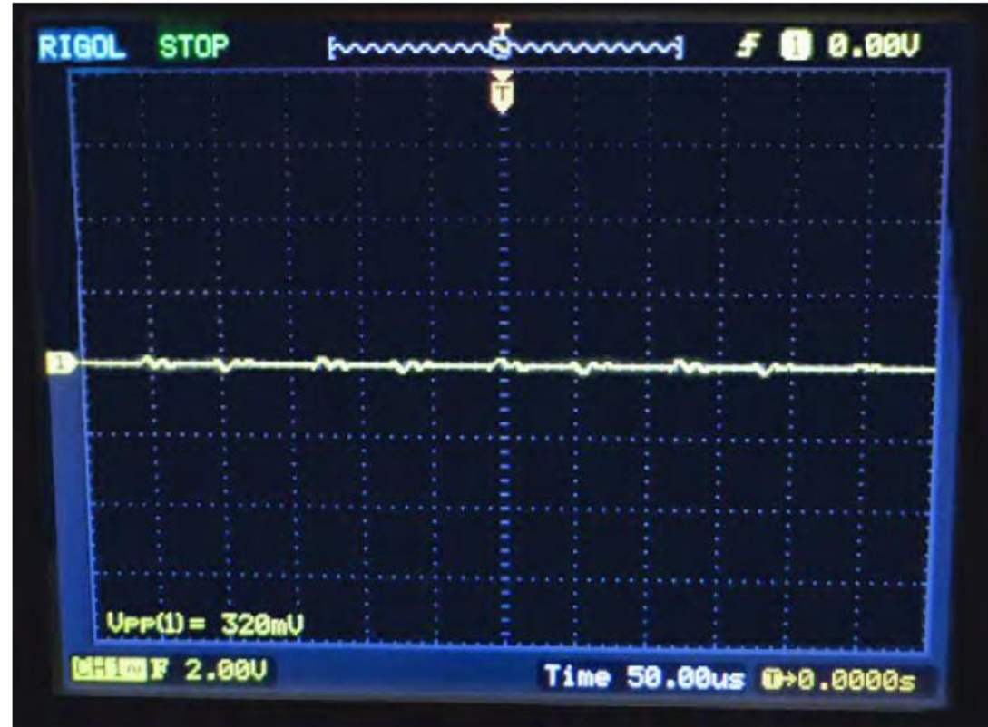
Shaft Voltage BPK
