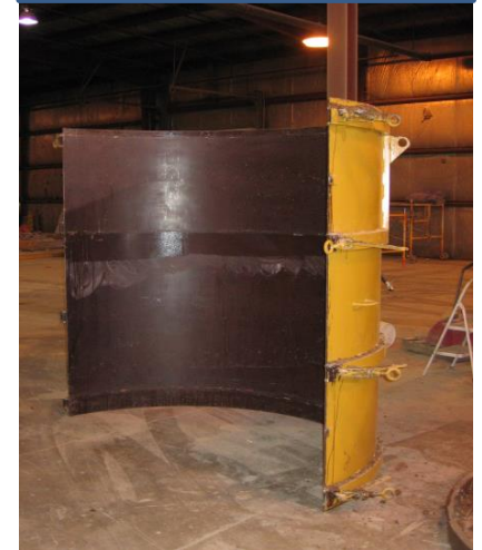
Outside form jacks (half side)
