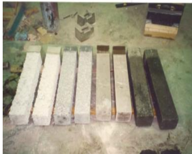
Figure 5.3 PCC and SFC beams after 90 days of exposure to H_2SO_4
