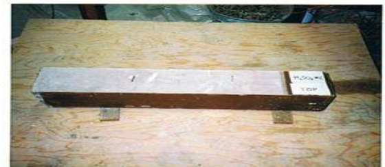
Figure 5.4 ICOM beam after 90 days of exposure to H_2SO_4
